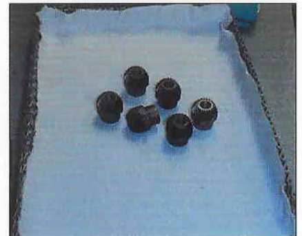
Fig 5 — Production lots of small gears have now been low-pressure carburized using experimentally determined settings. Case depth and surface hardness have been within acceptable tolerances.
