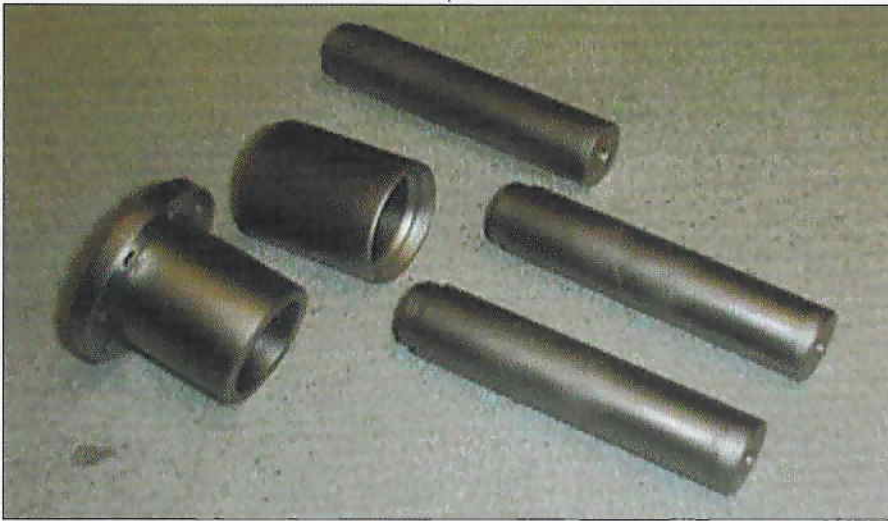
Figure 2 — Tool steel bearing components, as vacuum tempered to a bright finish.
